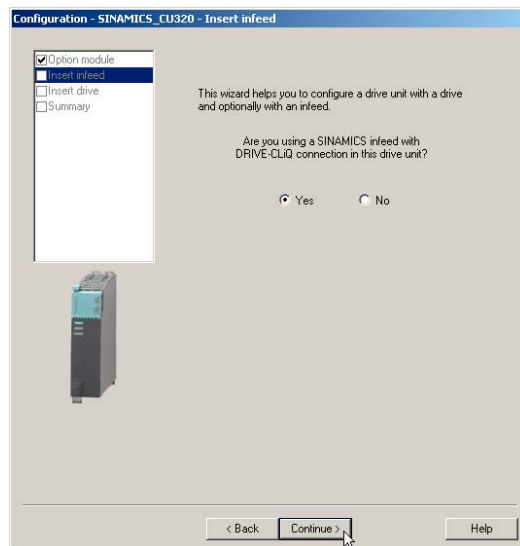
Fig. 3-16 Configuration – Introduction to SINAMICS CU320
